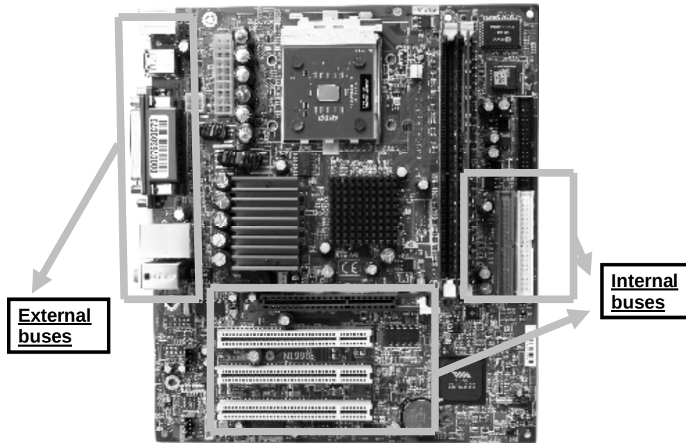
Fig. 2.6. Position of computer buses on the motherboard
