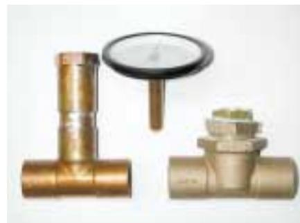
A brass seat tee with reducer (right) keeps the thermometer sensor in the fluid's flow. Copper fittings (left) don't work as well.
